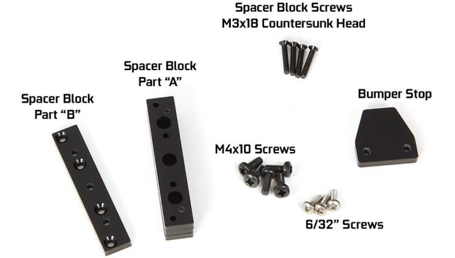
There are two ways to fix the bracket. First is to screw it directly to the Pci Slots, if your card is narrow you can use this option. The second, is to mount it on top of a 20mm spacer block. This will move the bracket closer to the side panel window in case you have a custom pcb card (which are usually quite large)
